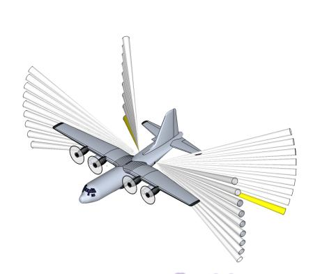
APAR single forward angle as it appears coming from the 4 APAR array faces. Maximum radar range ~75km depending on attenuation at C-band APAR combines reflectivity, velocity and dual-polarization measurements. Attenuation at C-band frequency is lower in heavy rain.
