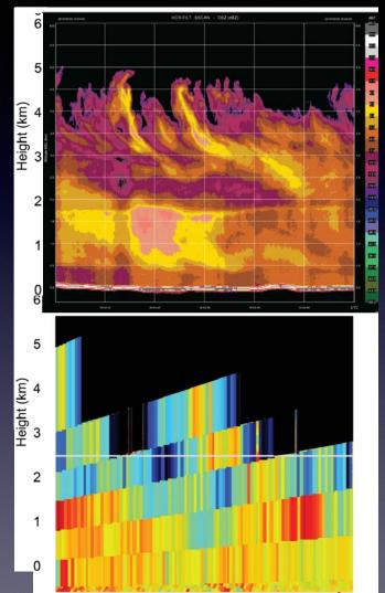
Reflectivity and Velocity measurements resolved wave structures and fine features in the same storm
